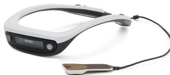
Figure 1. The PoNS™ device. The intraoral component of the system has a hexagonally patterned array of 143 gold-plated circular electrodes. This part of the device is held lightly in place by the tongue pressing toward the roof of the mouth, and rests on the anterior, superior part of the tongue. The intraoral unit connects to the controller module, which fits loosely around the neck.
