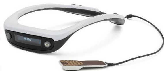
Figure 1. The PoNS™ device. The intraoral component of the system has a hexagonally patterned array of 143 gold-plated circular electrodes. This part of the device is held lightly in place by the tongue pressing toward the roof of the mouth, and rests on the anterior, superior part of the tongue. The intraoral unit connects to the controller module, which fits loosely around the neck.
